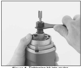
Figure 5. Tightening bit into router.
